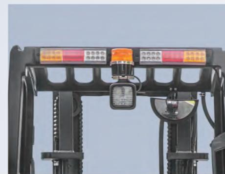
LED lights are used throughout the entire truck. The lights are energy efficient, have a longer service life, and offer a significant increase in performance.
