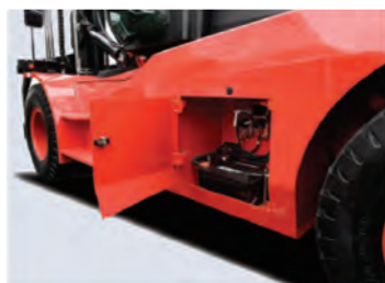
The battery compartment provides easy and convenient access to the battery.
