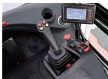
The Newly Designed LCD Instrument Display
