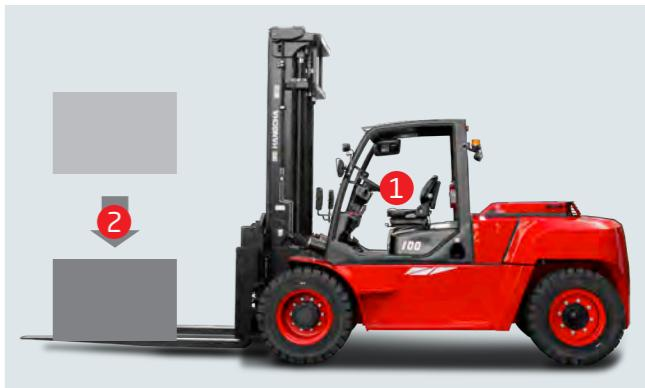
**1.** The Operator Presence Sensing System incorporates a lifting, tilting, and traveling stop function. When the operator leaves the seat, the system automatically locks the lifting/tilting functions and disables the forklift from traveling to ensure safety.
