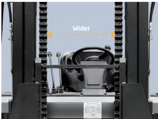
The mast was redesigned to provide broad forward visibility. This was done by relocating the hydraulic pipes of the fork positioner to the outside of the mast.
