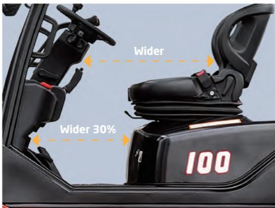
The foot space is now 30% wider to significantly reduce operator fatigue. The new wide, non-slip step makes getting in and out of the forklift safe and easy.
