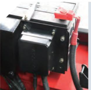
The controllers, relays, and safety fuses are all placed in the dust and water-free controller box. The main electronic components are also waterproof. This allows the operator to use the forklift in wet environments.
