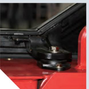
Dampening pads are placed where the chassis meets the steering axle, engine, torque converter, and overhead guard. The suspension seat also comes standard. This is all included in the design to reduce the amount of vibration to the operator and increase operator comfort.
