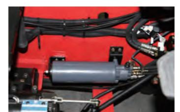
There's an energy accumulator in the braking system. This allows for the brakes to continue to function after the engine is shut off.
