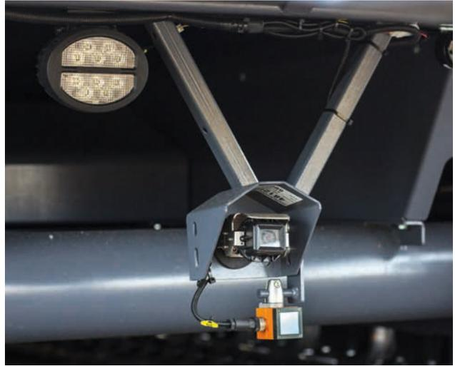
Synchronised speed: the distance sensor.
