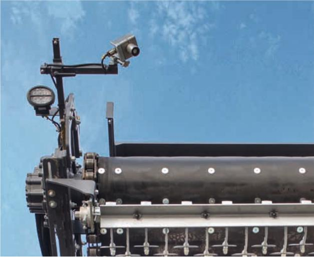
Automated material flow: the filling level sensor.
