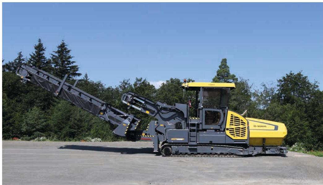
BMF 2500 S offset with slewing conveyor belt for the short version.
