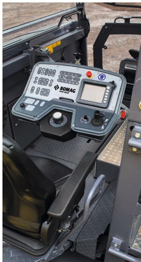
Comfortable: rotating seat with control panel.
