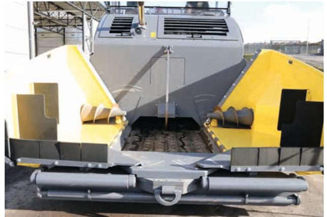
Two augers for homogeneous material flow.
