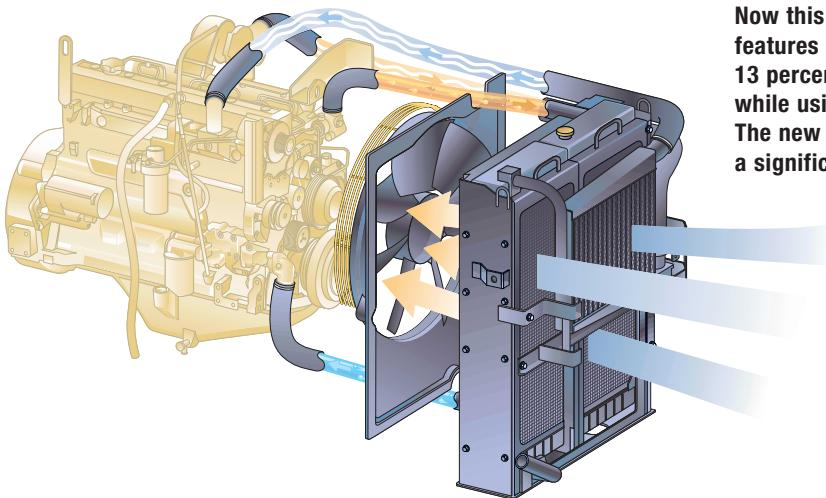
The cooling system's radiator is completely welded from the tube to the header joint, with a "square-wave" fin design to increase heat transfer by 18 percent.
