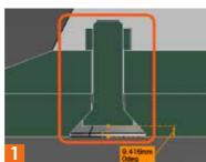
PLOW BOLT FOR CHANGEABLE PARTS New plow bolt will be applied on tooth adaptor and cutting edge
